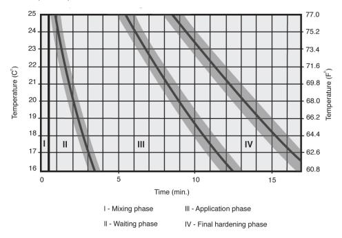
Handling and Setting Times vs. Temperature for vacuum mixing of Cobalt <sup>TM</sup> HV Bone Cement with Gentamicin (G-HV)
