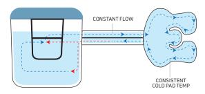
**The DonJoy**° **IceMan**° features a dual pump recirculation system that allows water warmed after flowing through the cold pad to be preserved and remixed with cooler ice water at a constant flow rate, providing consistent cool water distribution throughout the cold pad.
